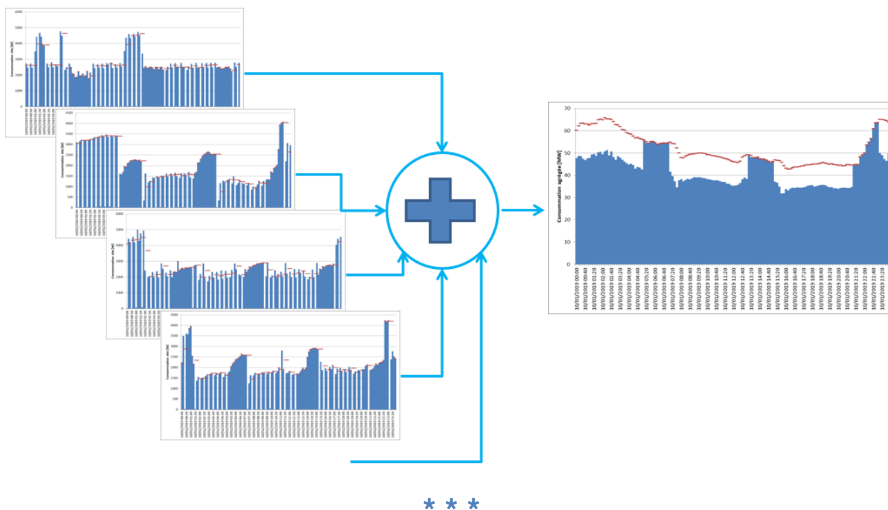
Illustration of the real-time individually determined baseline used for widespread DR involving short curtailments of numerous consumers' loads
